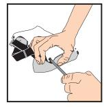
**6** Reattach Rubber Boot with screws.
